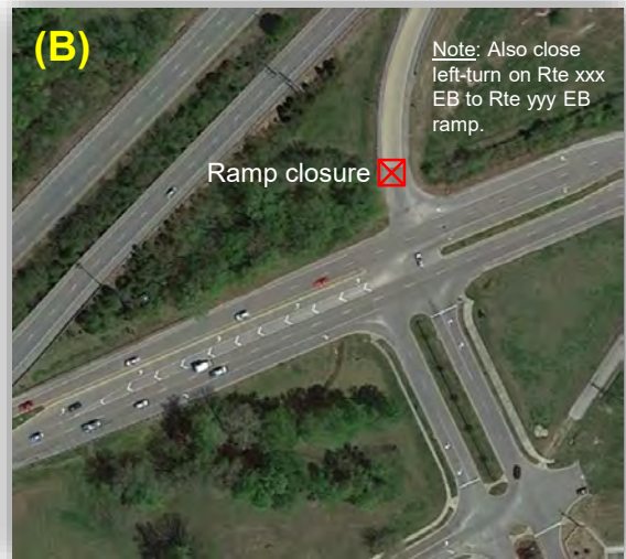
(B) A note for closing the left-turn lane on the cross road is provided (note the chevron marking).
