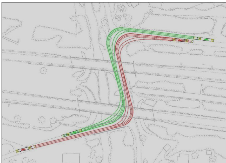
Figure 8: Route 609 Underpass Turning Radii
