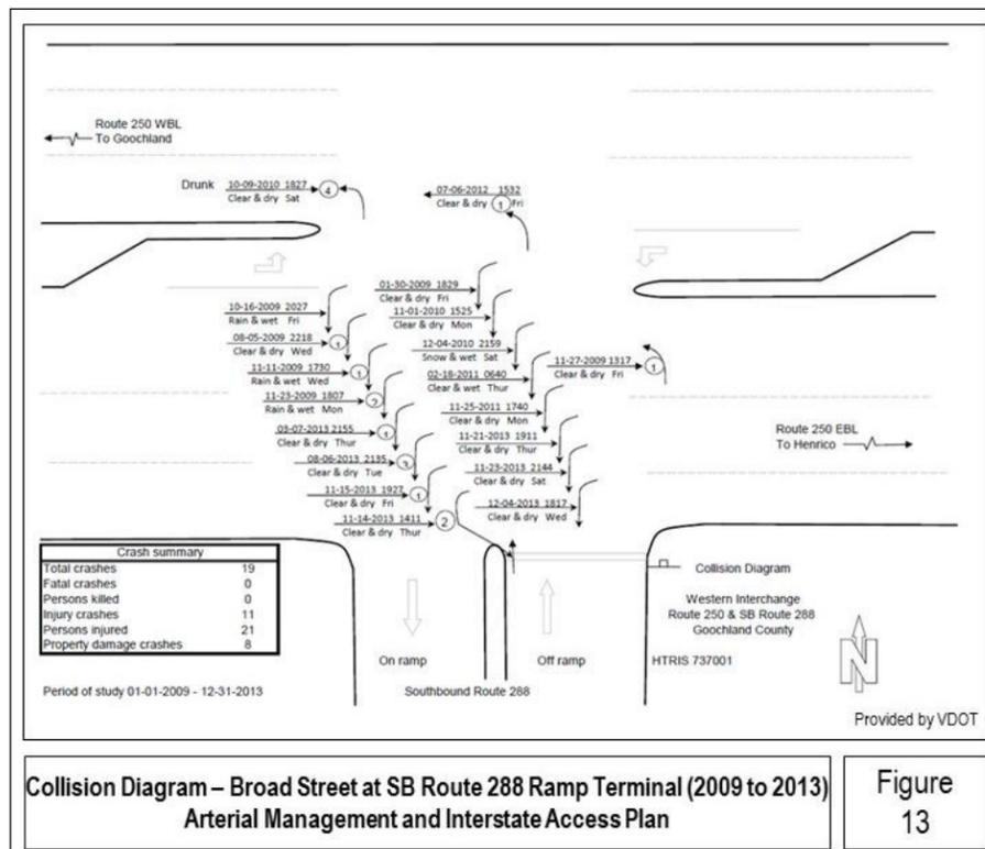
Collision Diagram - Broad Street at SB Route 288 Ramp Terminal (2009 to 2013)
