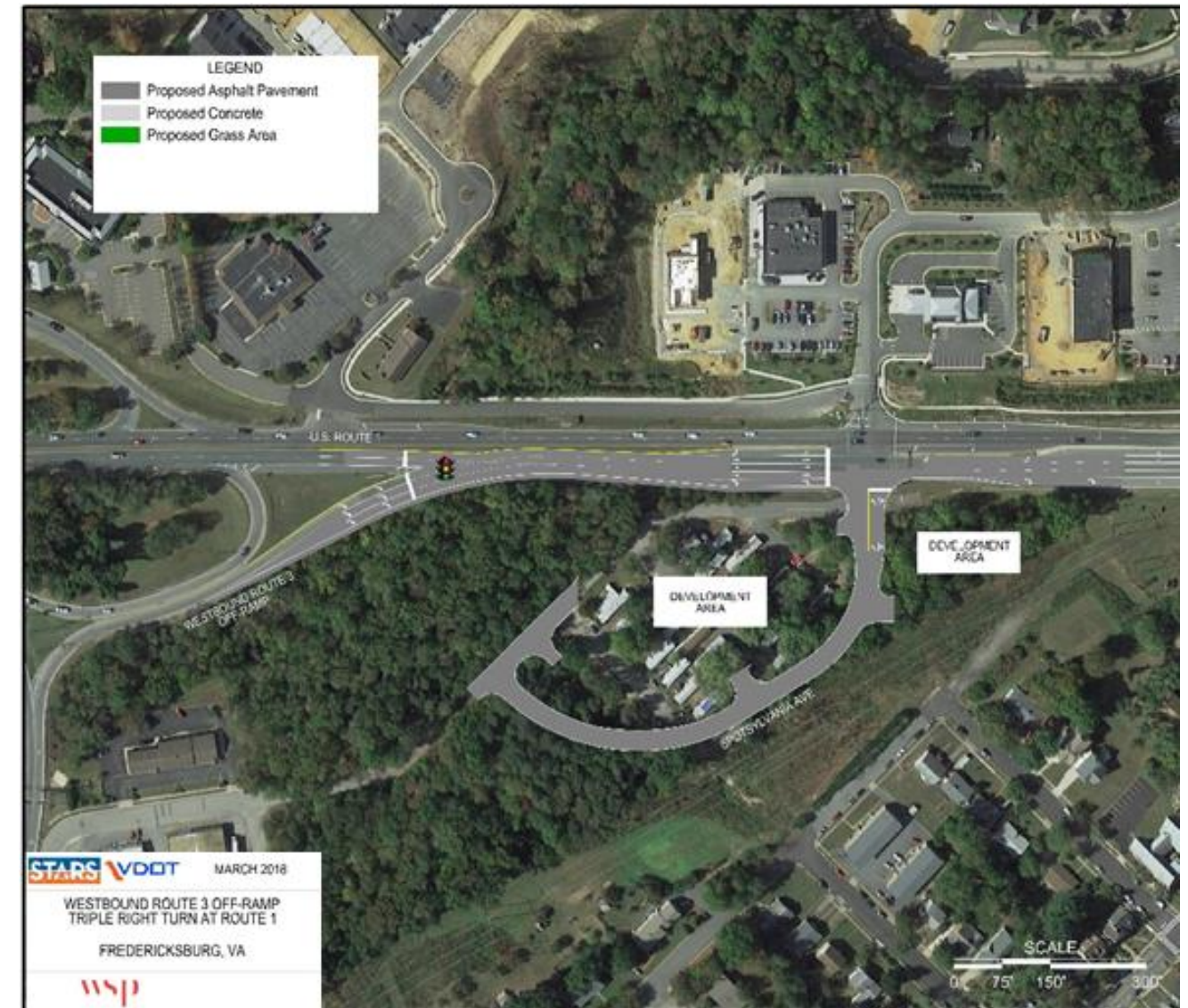
Figure 47. 2030 Preferred Alternative: Cowan Crossing/Spotsylvania Ave Intersection
