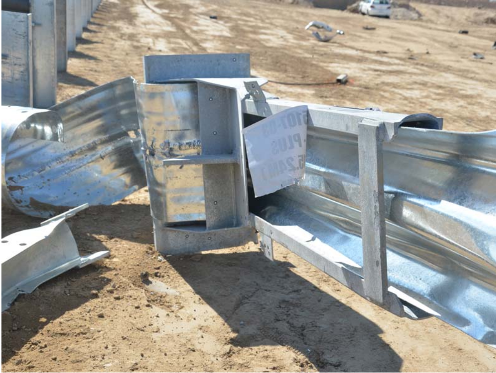
FIGURE 35. Test Article Damage
