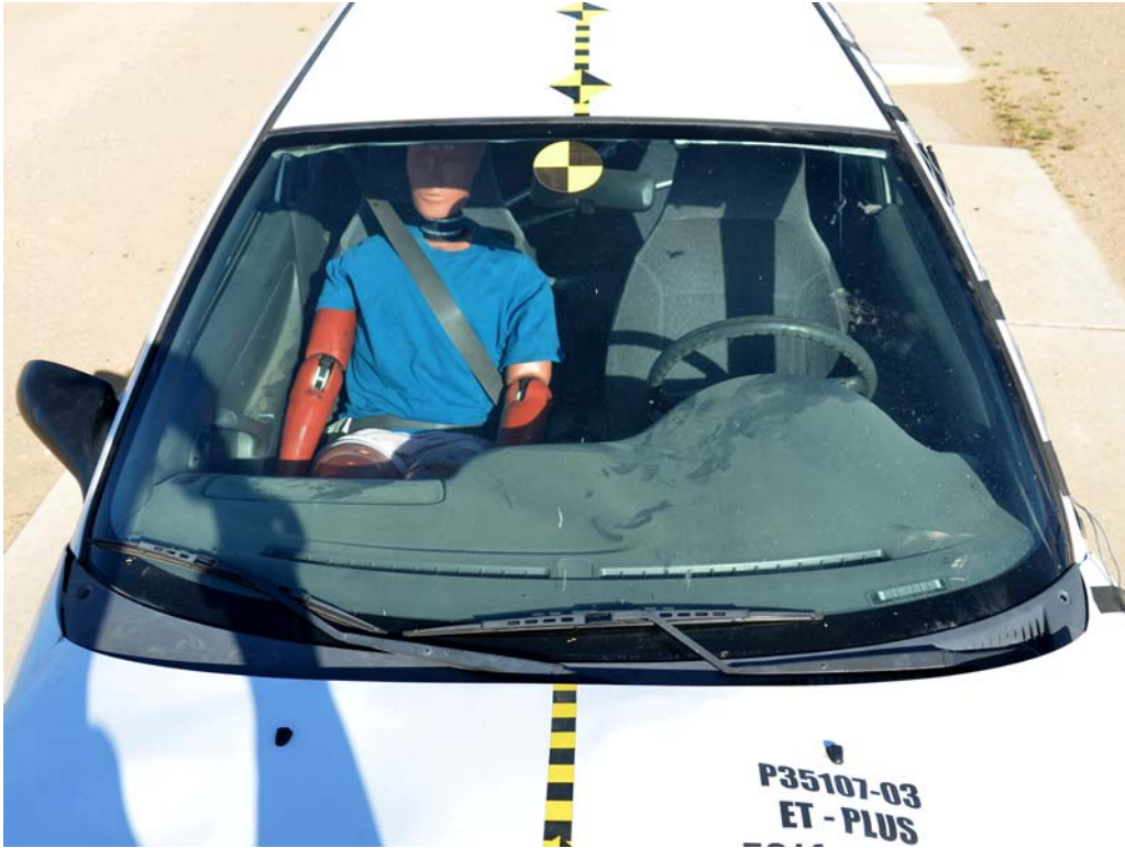
FIGURE 51. Post-Test View of Windshield
