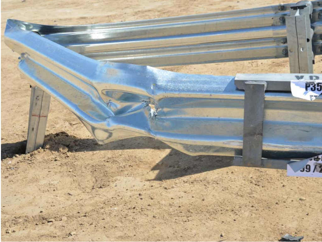
FIGURE 37. Test Article Damage
