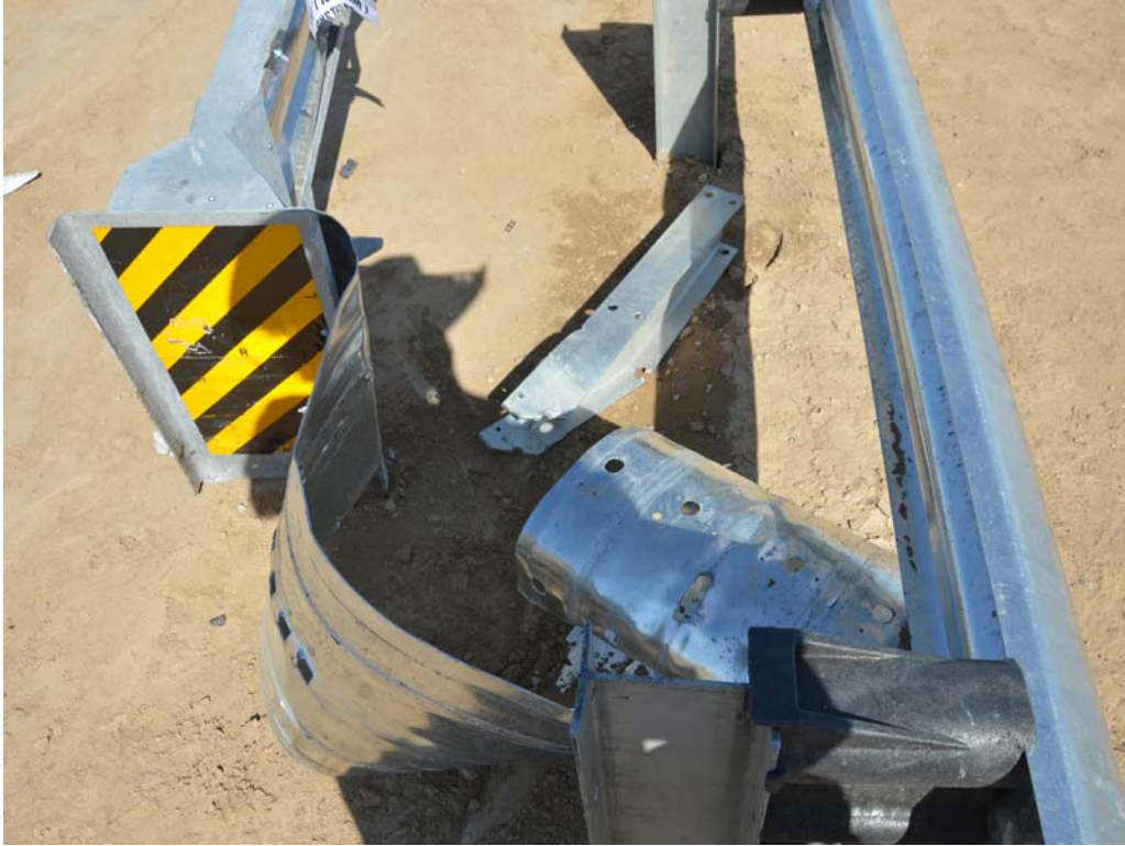
FIGURE 39. Test Article Damage
